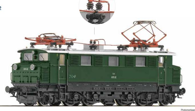
With its unusual axle arrangement (1A)'Bo(A1)', the locomotives of the 1670 class had a special position in the ÖBB vehicle fleet. The two middle driving axles are firmly mounted in the frame, the outer driving axles are combined with the neighbouring running axles to form a bogie.
