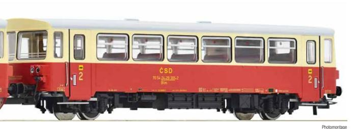
In order to replace the M 131.1 series railcars, which were no longer up to date, the Czechoslovak State Railways purchased new twin-axle diesel railcars with the series designation M 152.0. Delivered in series from 1975 onwards, these vehicles were powered by a 155 kW six-cylinder in-line engine and reached a top speed of 80 km/h. 56 seats were available in the passenger compartment.
